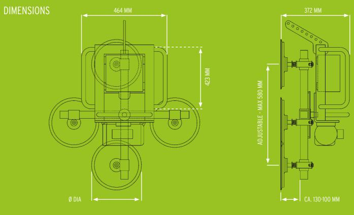
EV is a line of electric vacuum lifters powered by 400 Volt. The EV range is designed to lift airproof material of up to 600 kg in vertical position. The EV vacuum lifters are manufactured to be used internally in the production or in the warehouse and complies with EN13155-2003 standards.
