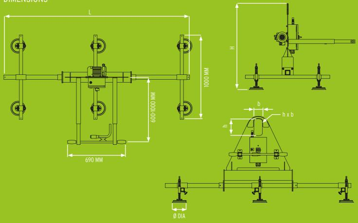
EH is a line of electric vacuum lifters powered by 400 Volt. The EH range is designed to lift airproof material of up to 2.300 kg in horizontal position. The EH vacuum lifters are manufactured to be used internally in the production or in the warehouse and complies with EN13155-2003 standards.
