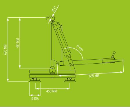
Type PN is a line of pneumatic lifters which are powered by compressed air. The PN range is designed to lift airproof material of up to 150 kg. All Vacuum lifters are lifting in either a horizontal position (PN-H), vertical position (PN-V) or are equipped with pneumatic tiltfunction (PN-VH). The lifters are manufactured under EN13155-2003 standards for vacuum lifters which are used internally in the production or in the warehouse.
